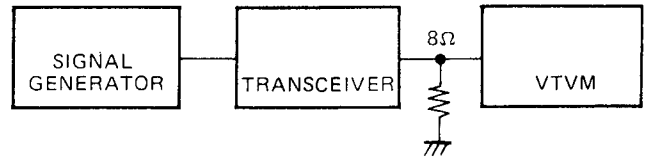
RX SENSITIVITY TEST SETUP
